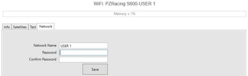
From the software, in the Network tab, it is possible to change the last part of the network name (USER 1) and the password. Once modified it will be necessary to close the RacePro program, turn off and on the GPS receiver.
